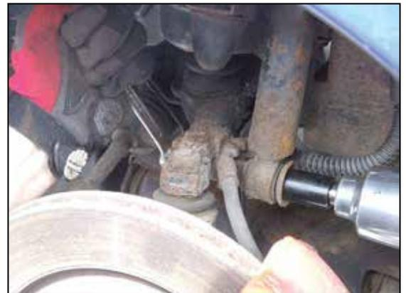
Figure 12, Note the correct positions of the brake hose clamp, spacer and two washers.
