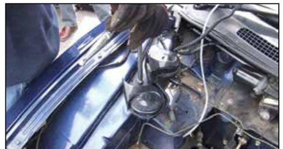
Figure 13, Remove horns and brackets.
