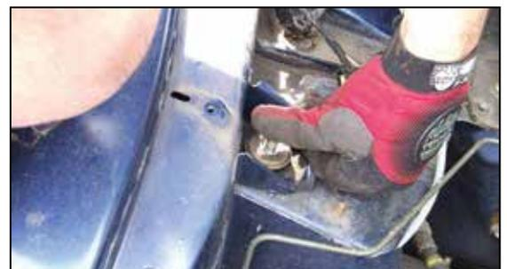
Figure 14, Remove the damper.
