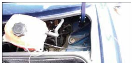
Figure 35, Move the coolant expansion tank.
