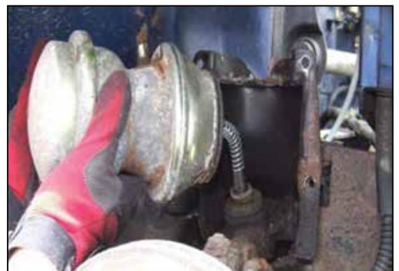
Figure 19, Gently pull displacer forward.
