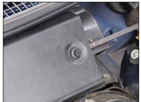
Figure 5, Prise out the rivet section.
