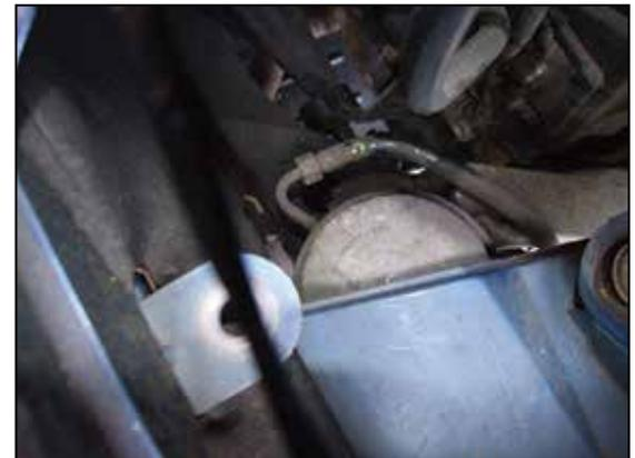
Figure 37, Remove the rear displacer.
