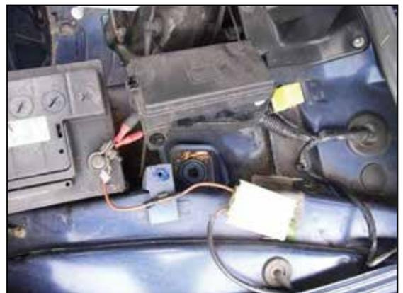
Figure 45, Move the under bonnet fuse box.
