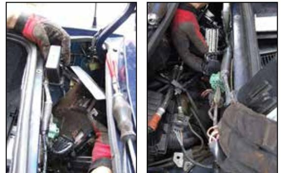
Figure 47-48, Disconnect the ECU connectors.
