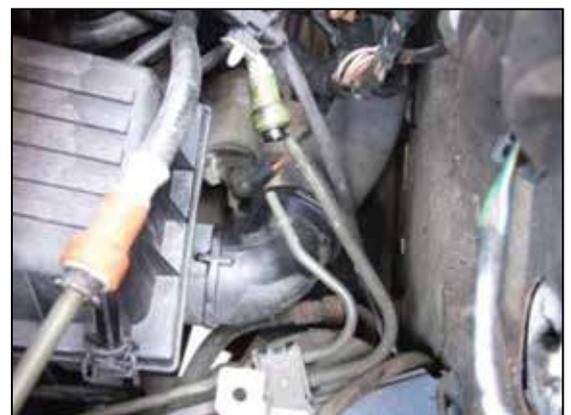
Figure 49, Air filter - single entry hose.
