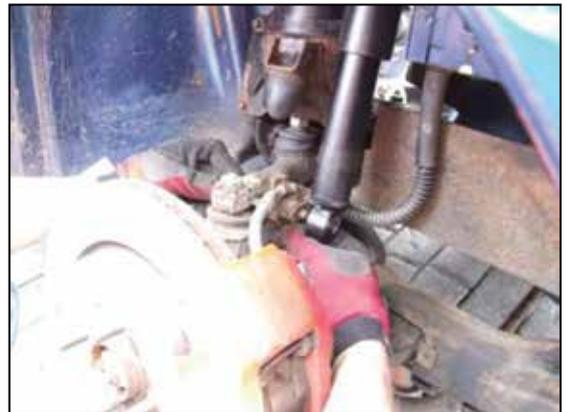
Figure 31, Refit the lower damper bolt.
