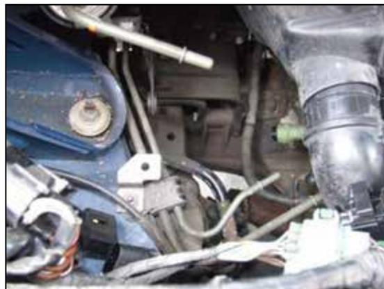
Figure 50, Air filter - dual entry hose.
