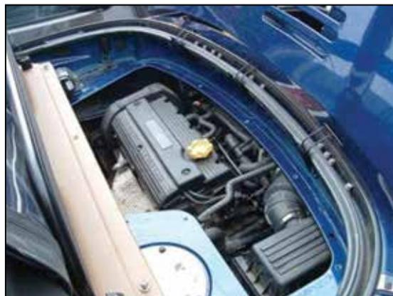
Figure 52, Remove engine cover.
