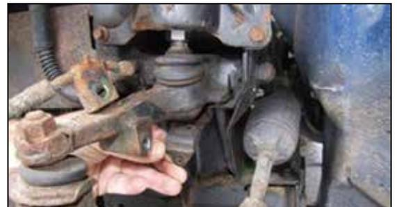
Figure 26, Adjuster, wound out by 18 turns.
